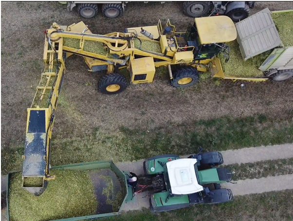
Separation of field and road transport during maize harvest (Maïke Siekmann/Thünen-Institute)
