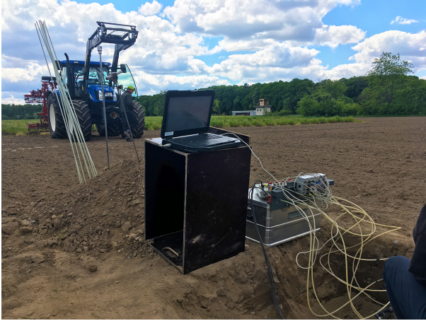
Demonstration of a soil deformation measurement (Susanne Döhler/UFZ)
