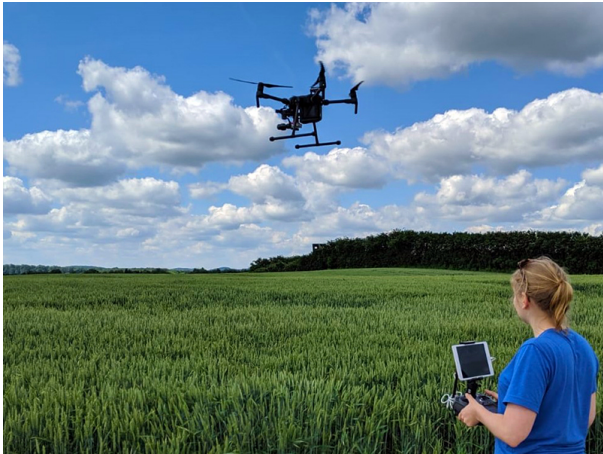
Field measurements with RGB and multispectral cameras (Fritjof Busche/CAU Kiel)
