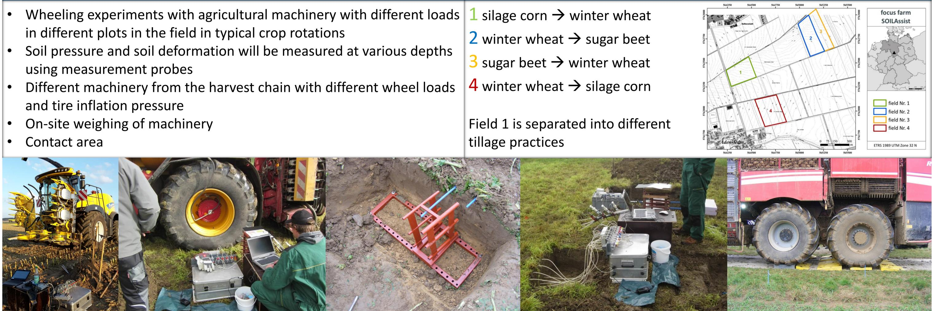
Soil pressure and soil deformation (depth: 20 cm) during repeated wheeling (2 axles) on a ploughed field
